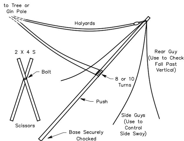
**Fig 13—Pulling on a gin line fastened slightly above the center point of the mast and on the halyards can assist in erecting a tall mast. The tensions should be just enough to keep the mast in as straight a line as possible. The "scissors" may be used to push on the under side and to serve as a rest if a pause in raising becomes necessary.**
